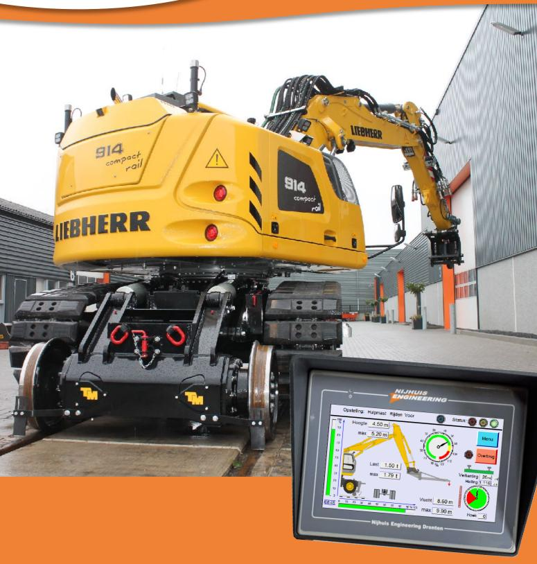
Rated Capacity Limiter for hi-rail excavators conform EN 15746
